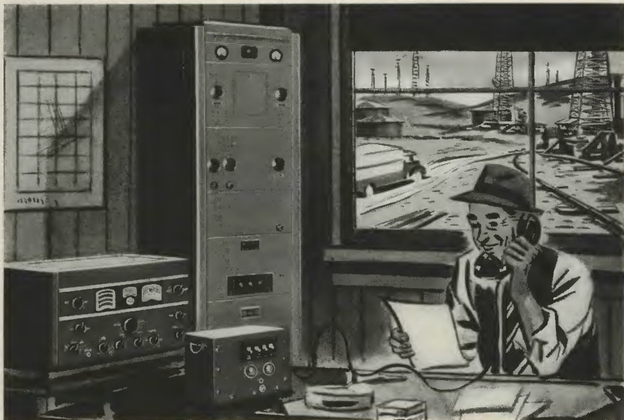
Illustrated is RCA type ET 4339, 200 watt 1.7 mc to 20 mc single or dual channel telephone or telegraph transmitter including remote control, and RCA type AR 88, .550 mc to 32 mc de luxe communications receiver.
